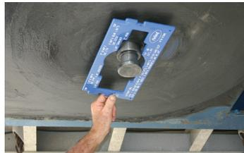
**Figure 4. Check for kingpin wear.**
