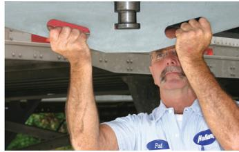
**Figure 1. Check upper coupler plate flatness.**
